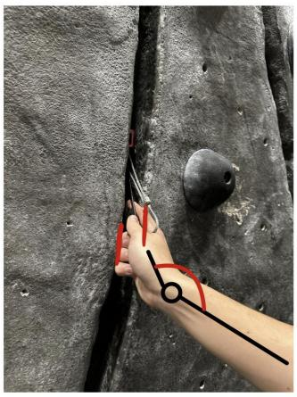
As tool is placed into crack it forces wrist flexion at uncomfortable angle, outside of neutral position
